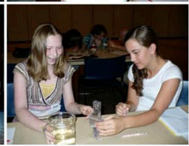
Students analyze the density of water and alcohol to determine the mix required so that an ice cube has neutral buoyancy.
