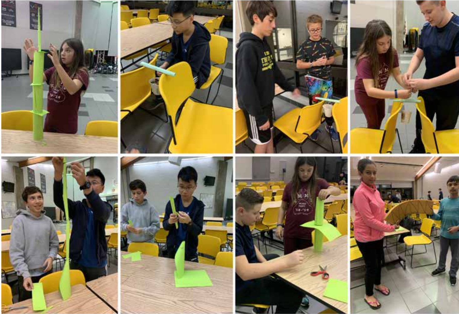
We experimented to determine which shape is strongest: a solid beam or a tube. The tube won.
